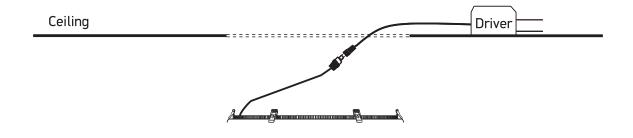
C Install fitting using springs supplied.
