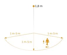
Possible mounting height: 1,80 m – 2,00 m Orange: radial and tangential 3 scalable axes
