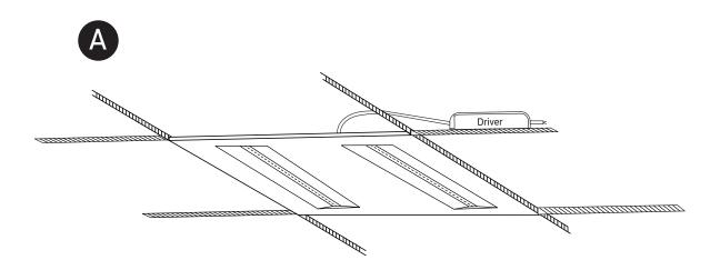
Recessed fitting for 600x600mm T-rail false ceilings.
