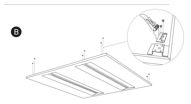
Ceiling mount suspended applications using optional kit 050108A.
