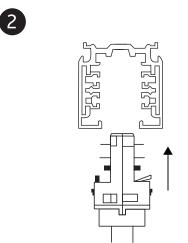
When installing the adaptor into the track, ensure that it is orientated correctly.
