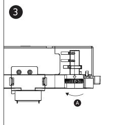
Rotate selector knob  $oldsymbol{\mathbb{A}}$  to the desired position circuit.
