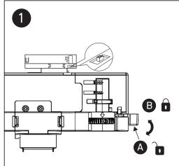
To mount the track adaptor into the track system, first check that the selector knob is at position (A) move to position **B** to lock the adaptor.
