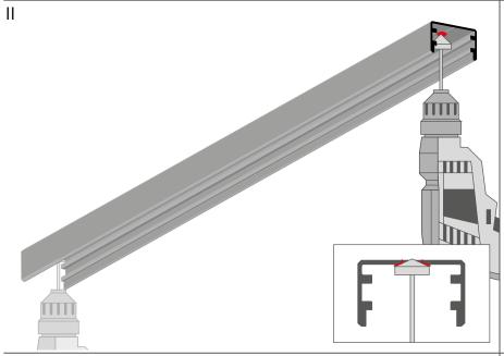
Chamfer the fastener holes.
