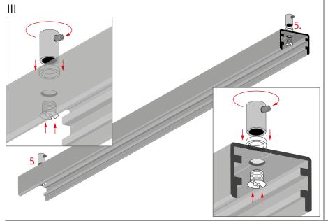
Screw the fasteners (5) to the profile.
