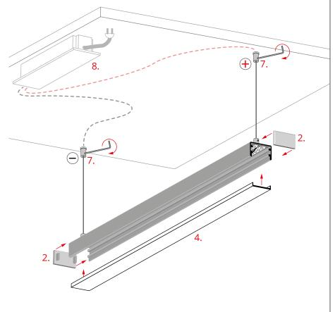
Mount the cover (4) and the end caps (2). Suspend the profile on the ceiling fasteners (7). Connect the 12 V / 24 V power supply (8) to the ceiling fasteners.
