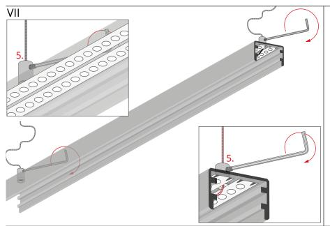
Lock the cables by tightening the pressure screws in the heads of the fasteners (5).
