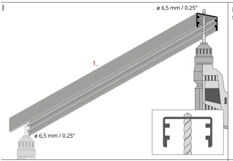
Drill holes in the profile (1) where the fasteners will be mounted.
