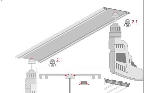
Countersink the screws (2.1) so they sit flush with the surface.
