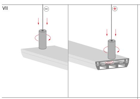
Insert the entire assembly into the sleeve and tighten the the fastener body.
