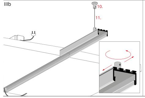
Connect the ceiling fastener (10) and the profile fastener with the wire (11).
