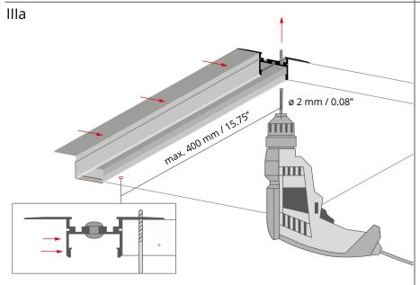
Place the profile on the edge of the drywall board and drill holes through the board and the profile's flange.
