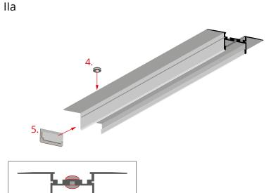
Attach the end cap (5) to the profile and install the gland (4) in the pre-drilled hole.
