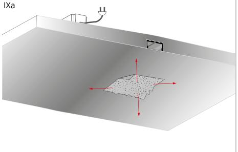
After the plaster has dried, sand the surface with sandpaper.
