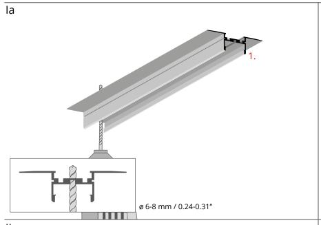
Drill a hole for the power cable in the GIZA-LL-UST (1) profile.
