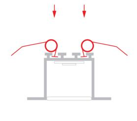
$\boldsymbol{2}_{\bullet}$  Insert the extrusion in the groove bending the spring arms towards each other.
