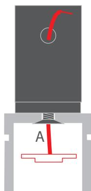
**6.** Mount the light fixture on the arm (E). Block the arm by tightening the pressure screw in the top head with the Allen wrench.
