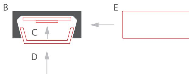
**3.** Connect power to the LED strip and mount the extrusion (B) in the mounting bracket.
