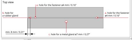
a. On both sides, from the side of the profile cross-section, thread the sockets for end cap bolts to a depth of approx. 15 mm / 0.59". (M3 tap)
