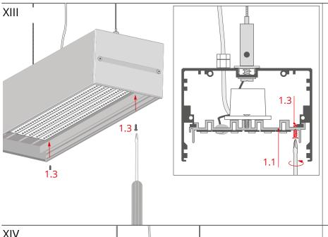
Secure the extrusion item (1.1) against slipping out by screwing the locking bolts (1.3) into the pre-drilled holes.
