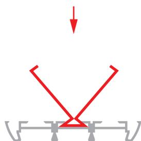
2. Drill a hole for mounting the extrusion.
