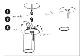
installation for 1.0 LED with blade springs
