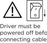
Driver must be powered off before connecting cables.
