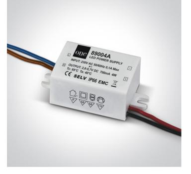
IP66 Constant current LED driver, non-dimmable for 700mA LED spots / LED fittings, 2-4W.
