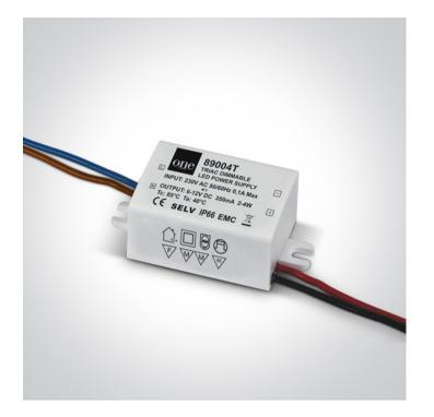
IP66 Constant current LED driver, Triac dimmable, for 350mA LED spots / LED fittings, 2-4W.
